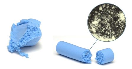
Glass microspheres are commonly used as an additive in resins, plaster and even concrete. The net effect is to provide a mechanism for introducing microscopic air bubbles and thus reduce density. Micromass can be mixed into practically any polymer-based or water-based material and actual applications range from the manufacture of low-density adhesives in model aircraft to floatable polymers in marine applications. The uses for micromass are many and varied, but include:
